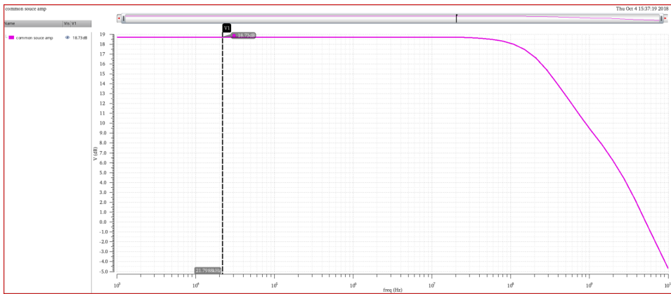
Figure 8: AC Gain Simulation Result of CS Stage
